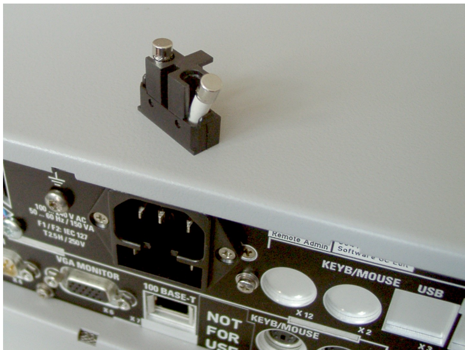
Figure 12.2: Exchanging Power Supply Fuses (2)
